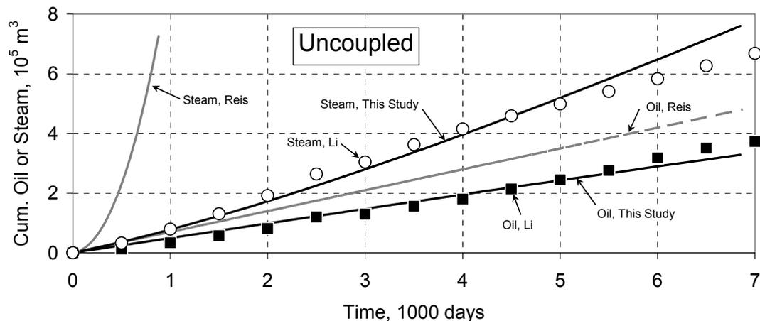
Figure 10. Comparison of numerical modeling results with two analytical uncoupled models
