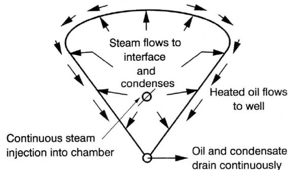
Figure 1. Steam Assisted Gravity Drainage (SAGD) process, from Butler (1991)
