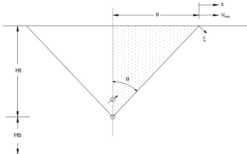
Figure 4. Geometry of steam chamber and its growth
