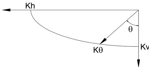
Figure 3. Elliptical relation between horizontal and vertical permeability
