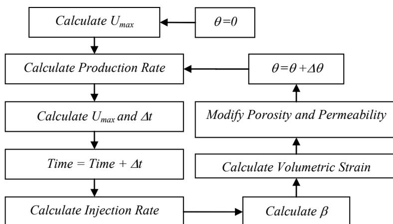
Figure 7. Solver flowchart
