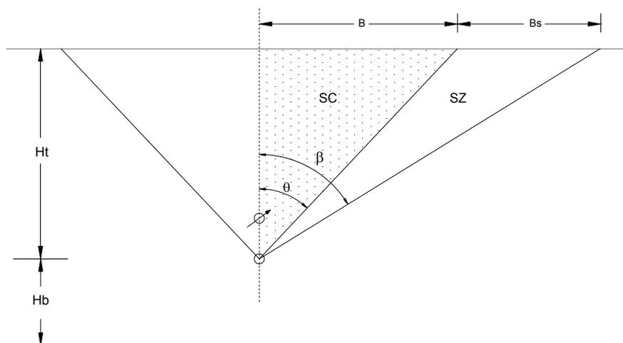
Figure 5. Moving shear zone in front of steam chamber
