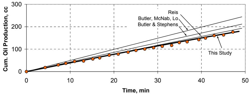
Figure 8. Comparison of measured and calculated model (Test 1)
