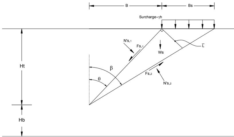
Figure 6. Effective forces on the wedge
