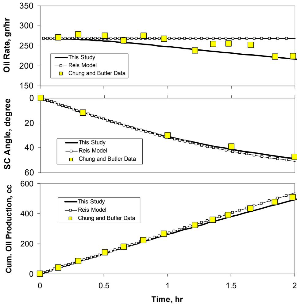
Figure 9. Comparison of measured and calculated model (Test 2)
