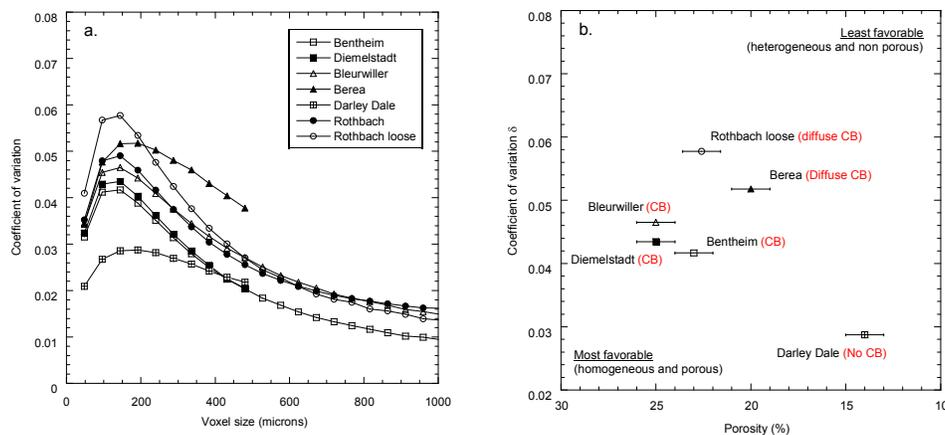
Figure 1. a. Average local  $\delta$  value as a function of voxel size in the sandstones studied. b. Type of compaction as a function of porosity and heterogeneity. Compaction bands develop in more homogeneous and more porous samples.
