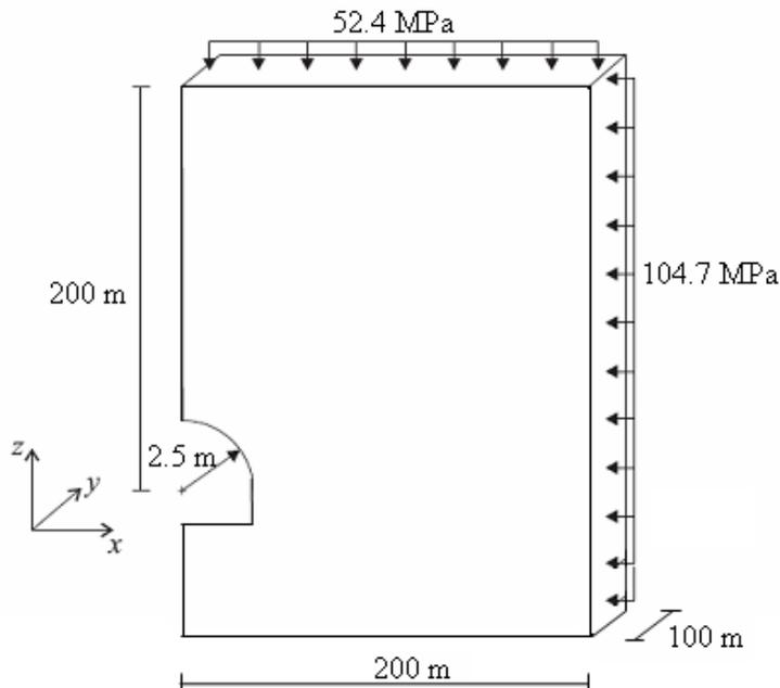
Figure 1. Geometry and loading of the FLAC<sup>3D</sup> model.
