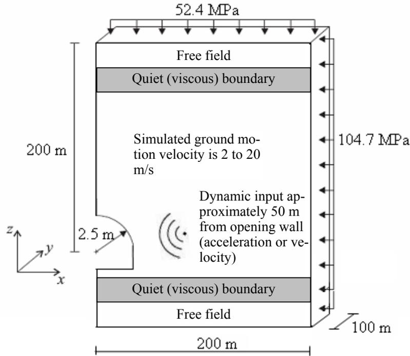
Figure 7. Geometry and loading of the FLAC<sup>3D</sup> model.
