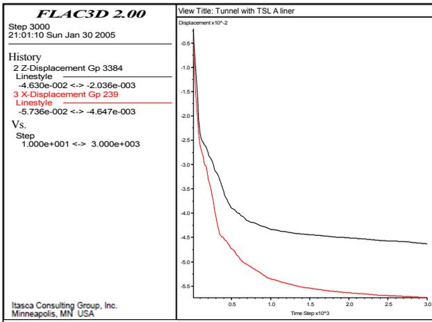
Figure 4. Displacement history plots versus time steps for tunnel with 3.5 mm (TSL A) liner.
