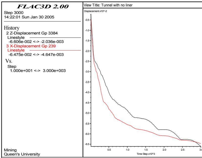
Figure 3. Displacement history plots versus time steps for tunnel with no liner.
