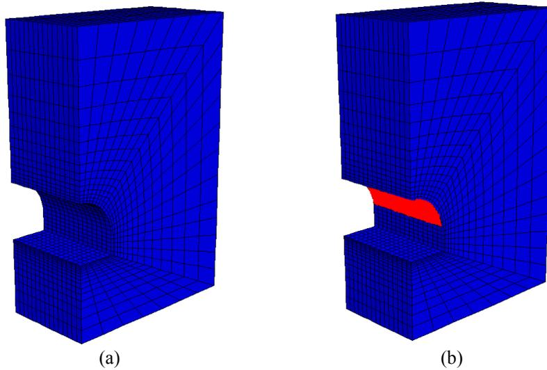
Figure 2(a). Tunnel with no liner, and (b). Lined tunnel.
