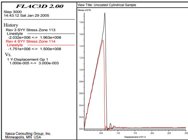
Figure 6. Stress-displacement plots for uncoated Mohr-Coulomb material.
