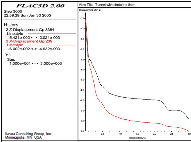
Figure 5. Displacement history plots versus time steps for tunnel with 10 cm shotcrete liner.
