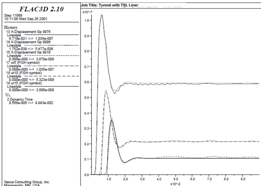
Figure 8. Displacement histories recorded up to 0.1 second at the tunnel surface.
