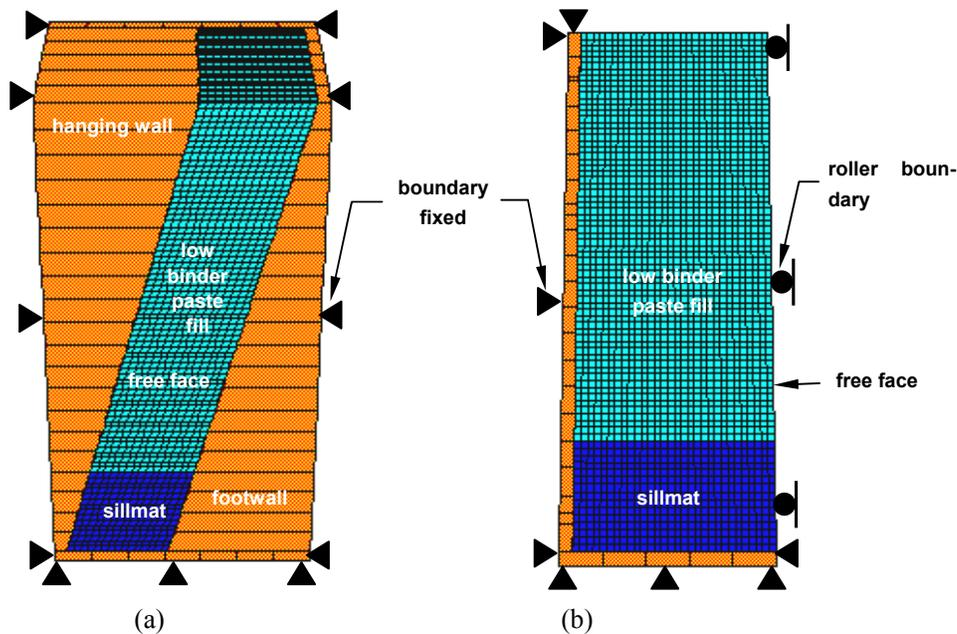
Figure 2 (a). 3-D paste fill free-standing height geometry. (b). Long section.
