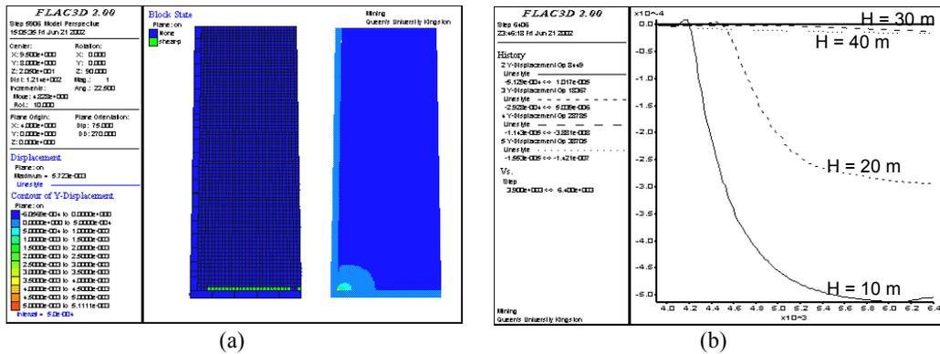
Figure 8 (a). Plastic state, displacement vectors and displacement contours in a long section for sillmat thickness equivalent to the stope width overlain by 2.5% paste fill blend cured for 28 days in a 7.5 m wide stope inclined at 60° with rough rock walls (shear-n=shear yielding now, shear-p=shear yielding in past); and (b). History of horizontal displacements (y-displacement) of the vertical fill face versus time step at heights 10, 20, 30 and 40 meters from fill base.
