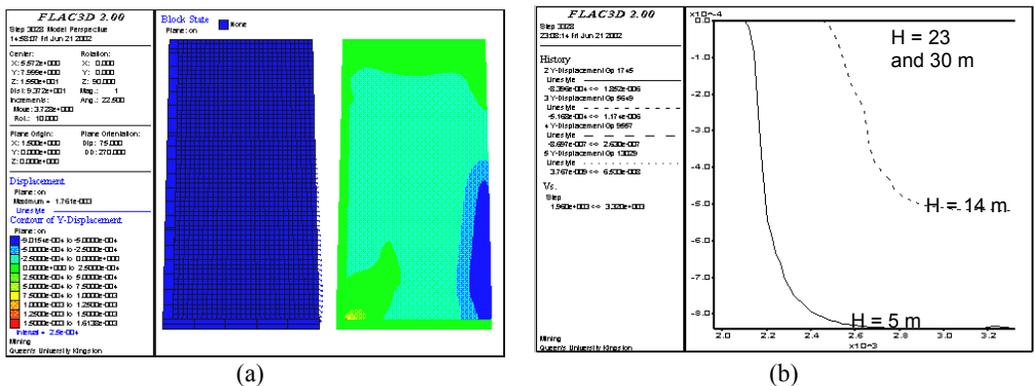
Figure 5 (a). Plastic state, displacement vectors and displacement contours in a long section for sillmat thickness equivalent to the stope width overlain by 2.5% paste fill blend cured for 28 days in a 3 m wide stope inclined at 60° with rough rock walls (shear-n=shear yielding now, shear-p=shear yielding in past); and (b). History of horizontal displacements (y-displacement) of the vertical fill face versus time step at heights 5, 14, 23 and 30 m from fill base.
