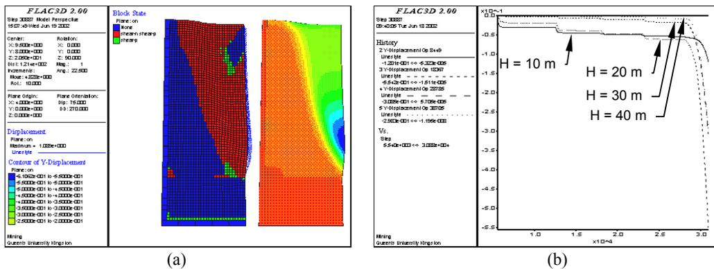
Figure 9 (a). Plastic state, displacement vectors and displacement contours in a long section for sillmat thickness equivalent to the stope width overlain by 2.5% paste fill blend cured for 28 days in a 7.5 m wide vertically inclined stope with smooth rock walls (shear-n=shear yielding now, shear-p=shear yielding in past); and (b). History of horizontal displacements (y-displacement) of the vertical fill face versus time step at heights 10, 20, 30 and 40 meters from fill base.
