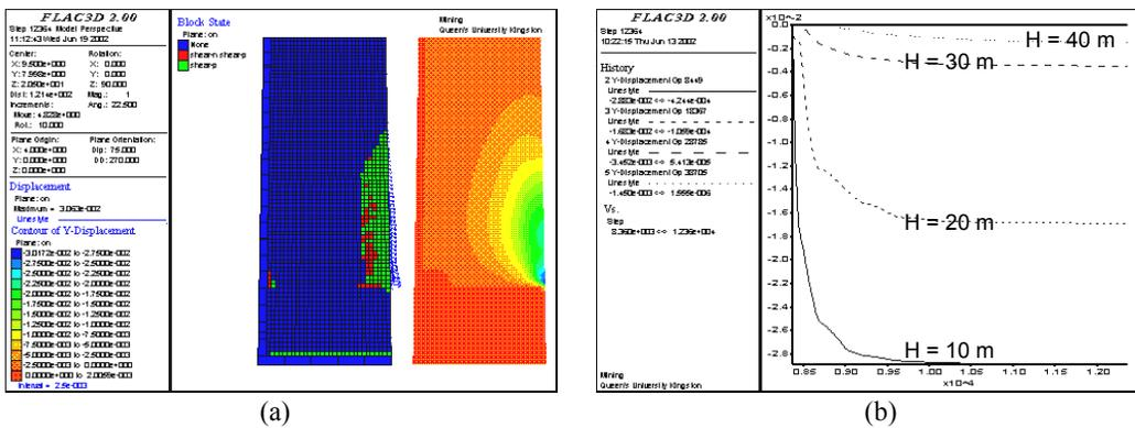
Figure 6 (a). Plastic state, displacement vectors and displacement contours in a long section for sillmat thickness equivalent to the stope width overlain by 2.5% paste fill blend cured for 28 days in a 7.5 m wide vertically inclined stope with rough rock walls (shear-n=shear yielding now, shear-p=shear yielding in past); and (b). History of horizontal displacements (y-displacement) of the vertical fill face versus time step at heights 10, 20, 30 and 40 m from fill base.
