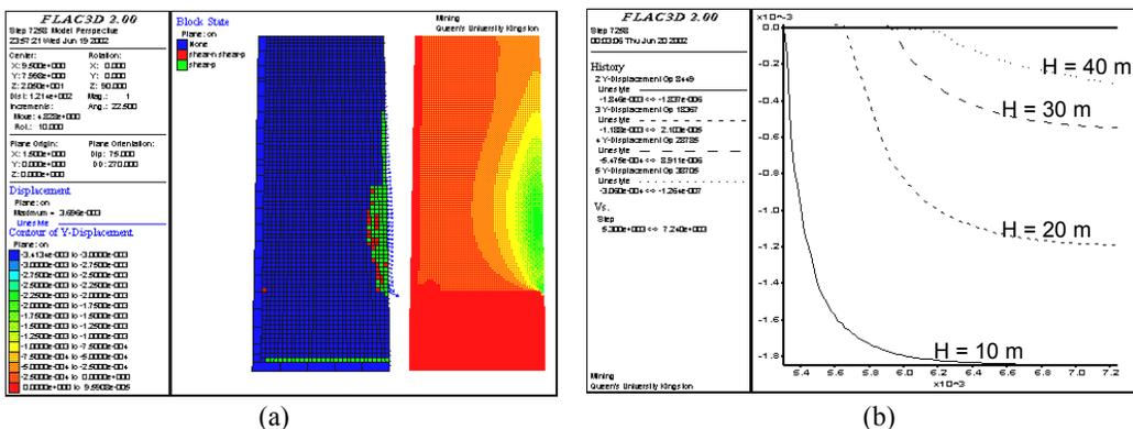
Figure 7 (a). Plastic state, displacement vectors and displacement contours in a long section for sillmat thickness equivalent to the stope width overlain by 2.5% paste fill blend cured for 28 days in a 7.5 m wide stope inclined at 75° with rough rock walls (shear-n=shear yielding now, shear-p=shear yielding in past); and (b). History of horizontal displacements (y-displacement) of the vertical fill face versus time step at heights 10, 20, 30 and 40 meters from fill base.
