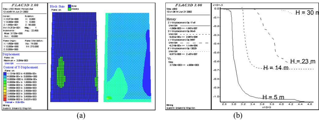
Figure 4 (a). Plastic state, displacement vectors and displacement contours in a long section for sillmat thickness equivalent to the stope width overlain by 2.5% paste fill blend cured for 28 days in a 3 m wide stope inclined at 75° with rough rock walls (shear-n=shear yielding now, shear-p=shear yielding in past); and (b). History of horizontal displacements (y-displacement) of the vertical fill face versus time step at heights 5, 14, 23 and 30 m from fill base.
