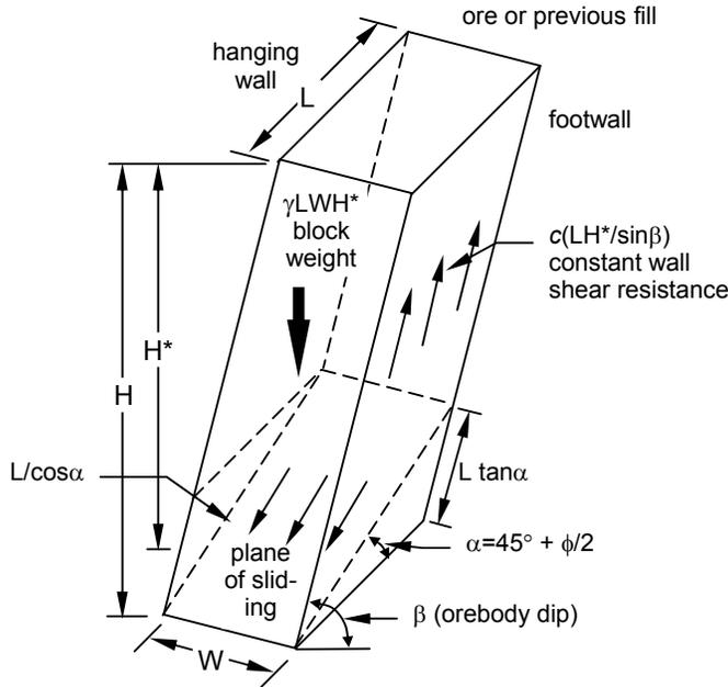
Figure 1. Confined block mechanism (adapted from Mitchell *et al*, 1982).
