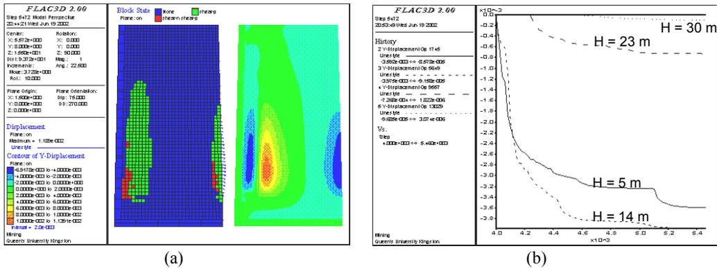
Figure 3 (a). Plastic state, displacement vectors and displacement contours in a long section for sillmat thickness equivalent to the stope width overlain by 2.5% paste fill blend cured for 28 days in a 3 m wide vertically inclined stope with rough rock walls (shear-n=shear yielding now, shear-p=shear yielding in past); and (b). History of horizontal displacements (y-displacement) of the vertical fill face versus time step at heights 5, 14, 23 and 30 m from fill base.
