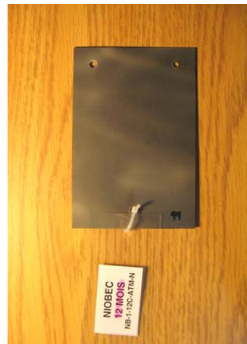
Figure 2. a) Configuration of the corrosion coupons with identification tag and b) corrosion coupon
