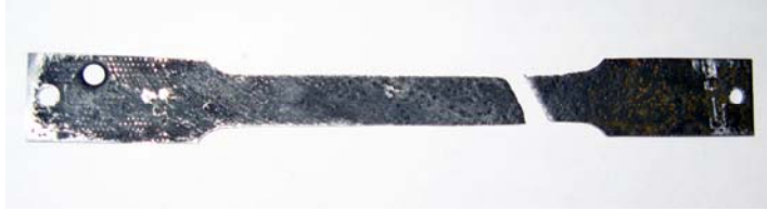
Figure 6. Coupon from Mine #4 site #2 after testing.
