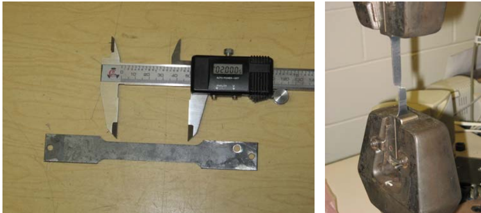
Figure 4. a) Tensile sample from a coupon and b) sample after testing
