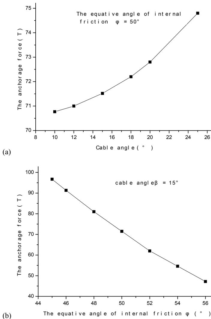
Figure 3. Relationships between: a) anchor force and cable angle; and b) anchor force and friction angle.
