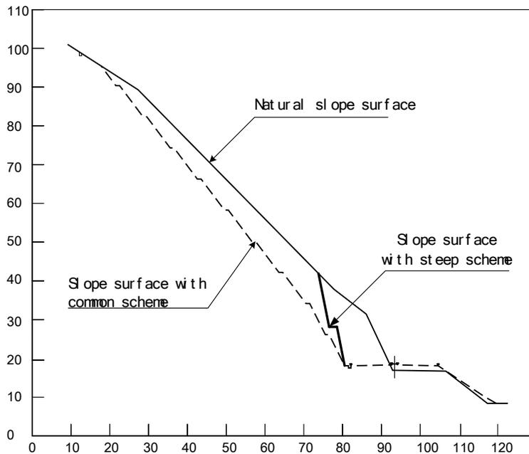
Figure 1. Illustration comparing the cut slope profiles for the common and steep design schemes.
