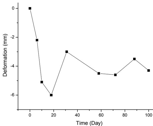
Figure 4. Horizontal deformation response of cut slope.
