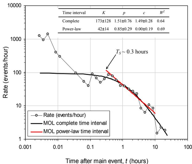
Figure 2. Determined MOL parameters using the complete and power-law time intervals.
