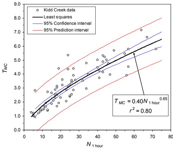
Figure 6. Relationship between  $T_{MC}$  and  $N_{1 \text{ hour}}$  for the Kidd Creek site.
