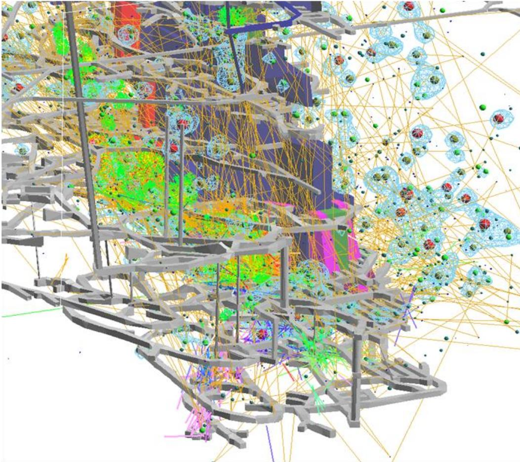
Figure 3. Seismic data processing and interpretation showing time (linkage lines) and source parameter relationships (colour/size) between mining induced seismic events – This is the researcher’s viewpoint.
