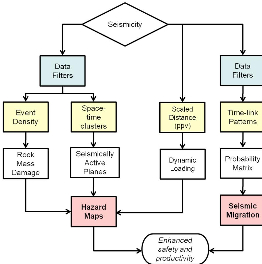
Figure 2. MIRARCO seismic data processing procedure chart, hazard factors and time-link logic are handled as two separate tasks
