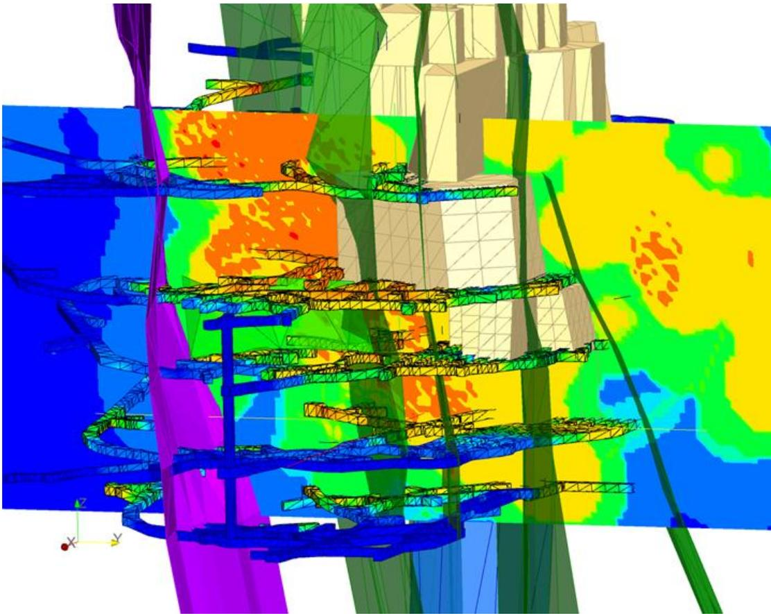
Figure 4. ParaviewGeo visualization of the Seismic Excavation Hazard Map showing a section and hazard projected onto mine excavations. This is the mine operator's viewpoint.
