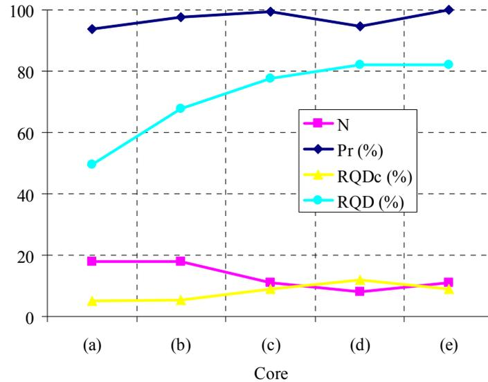
Figure 5. Rock mass quality description of the cores shown in Figure 4 with the new definition of  $RQD_c$  and the original definition of RQD.
