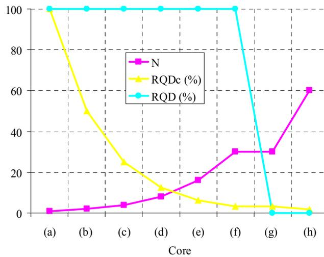
Figure 3. Variation of rock mass quality with the new definition of RQD<sub>c</sub> and the original definition of RQD for cores shown in Figure 1.
