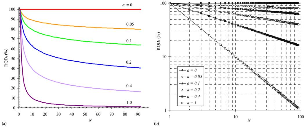
Figure 2. Variation of RQD<sub>c</sub> with number of pieces N using different values for parameter a, which varies from 0 to 1.0 ( $p_r = 100\%$ ): (a) in normal plane; (b) in log-log plane.
