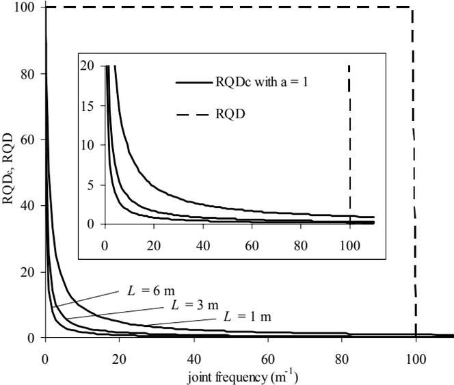
Figure 7. Variation of RQD with idealized joint frequency.
