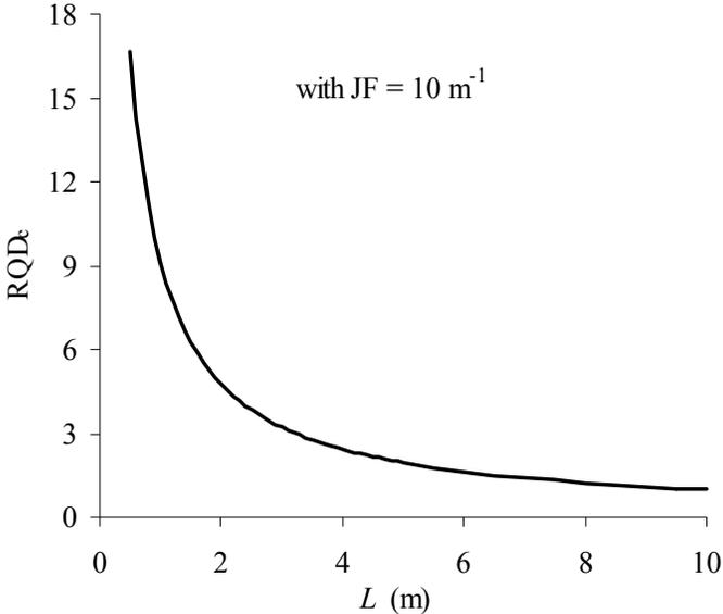
Figure 8. Scan interval or scale effect on the  $RQD_c$  value.
