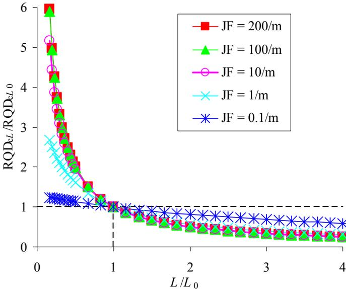
Figure 9. Variation of the normalized  $RQD_{cL}$  with the normalised scan interval  $L$  with different joint frequencies.
