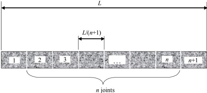
Figure 6. A fictive core with idealized uniformly distributed joints.
